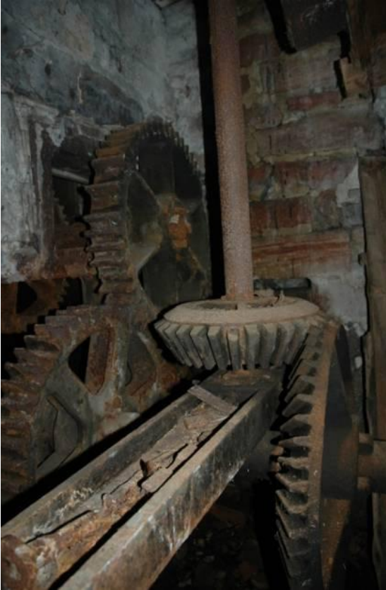
Bevel gear driving a vertical shaft
